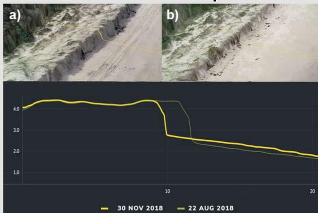
A 20 m cross-section comparison of storm damage at Inverloch over a 4-month period a) August 22<sup>nd</sup> 2018, b) November 30<sup>th</sup> 2018. Over this time, over 1.5 m has been lost from the dune face, but the height of the beach in front of the dune has increased by approximately 20 cm.
